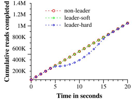
Figure 5: Effect of killing servers on throughput.
